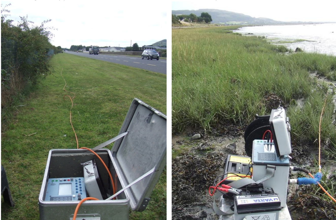
Figure 5.3: Terrestrial ERT surveying (a) roadside at Rockmarshall, Cooley Peninsula and (b) shoreline at Bellurgan.
