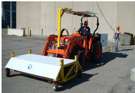
Ground survey of a nuclear facility to locate and identify contaminated particles
