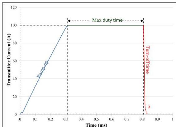
Figure 3: Transmitter waveform showing the ramp-up, maximum duty time, and turn-off times. Exact turn-off time is undetermined.
