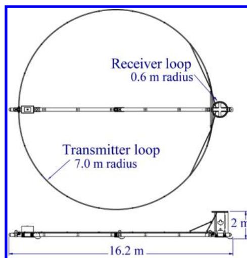
Figure 2: Concept drawing of the HTEM system currently under development. The transmitter is a single-turn 7 m radius loop with a moment of 15,400 A/m<sup>2</sup>. The receiver location has not been finalized yet. It is shown here offset and slightly elevated from the transmitter.
