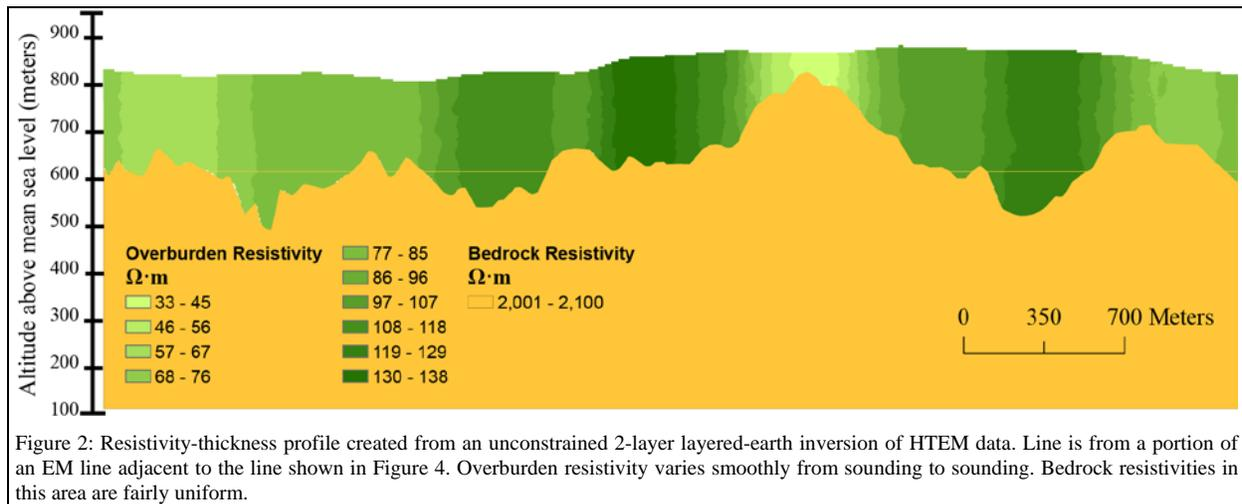
Figure 2: Resistivity-thickness profile created from an unconstrained 2-layer layered-earth inversion of HTEM data. Line is from a portion of an EM line adjacent to the line shown in Figure 4. Overburden resistivity varies smoothly from sounding to sounding. Bedrock resistivities in this area are fairly uniform.
