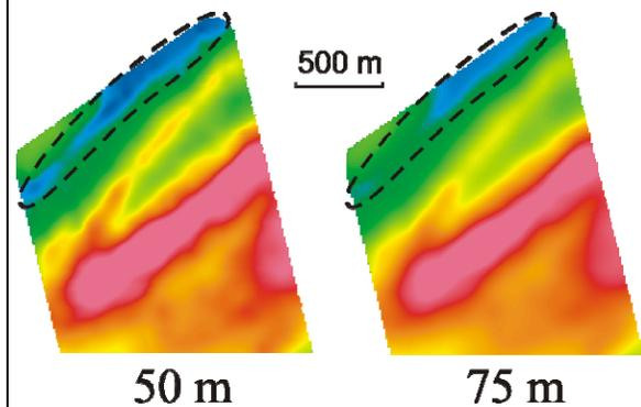
Figure 6: Detailed TMI maps of the sUAS data at 50 m altitude, and upward continued to 75 m altitude. Only the northern section of the survey area is shown. The magnetic valley, at the top of the map, is no longer identifiable as a linear trend at an altitude of 75 m. The colour scale is the same as in Figure 3.
