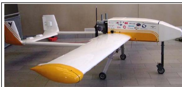
Figure 1: UAS prototype GeoSurv II is a twin-boom pusher aircraft with a wingspan of 4.9 m. The yellow pods at the wingtips house the magnetometers which are separated by 4.67 m. The UAS is designed for a flight endurance of 8 hours at 30 m/s. The landing gear can be replaced with a track for use with a catapult to enable flying in remote locations that do not have airstrips.
