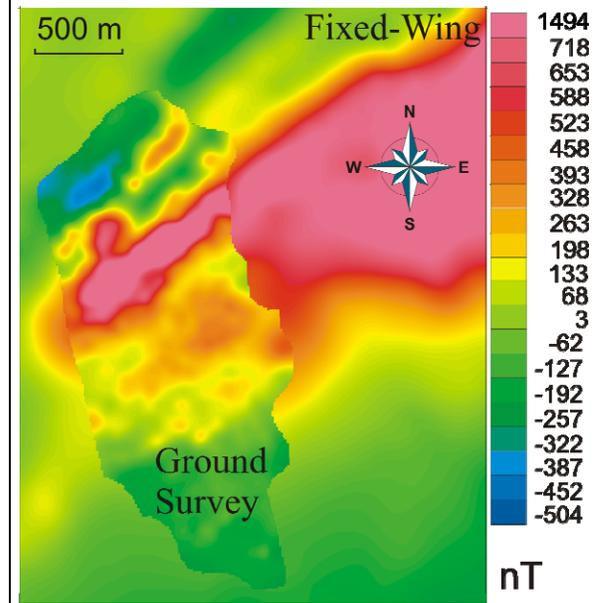
Figure 4: TMI map of the conventional fixed-wing survey data in the background and the ground survey, upward continued to 50 m, in the foreground.
