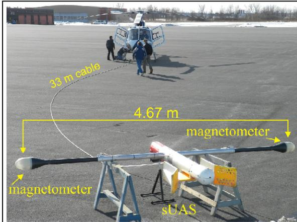
Figure 2: Heliported sUAS, a modified aeromagnetic bird with two cesium magnetometers laterally separated by 4.67 m. The sUAS was constructed for testing components such as the magnetometers, the magnetic gradiometer, and the obstacle detection and avoidance system. The center body is capable of housing instruments, and camera mounts have been added for bifocal video recording.
