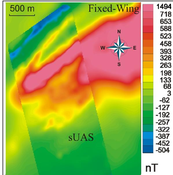
Figure 3. TMI map of the conventional fixed-wing survey data in the background and the sUAS data in the foreground. The fixed-wing survey was flown at an altitude of 150 m while the sUAS survey was flown at 50 m. The colour scale is the same as in Figure 4.
