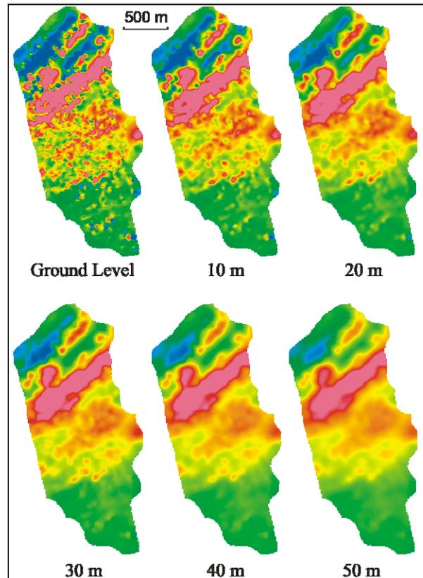
Figure 5. TMI ground survey maps that have been progressively upward continued from ground level to an altitude of 50 m in steps of 10 m. The colour scale is the same as in Figure 3.
