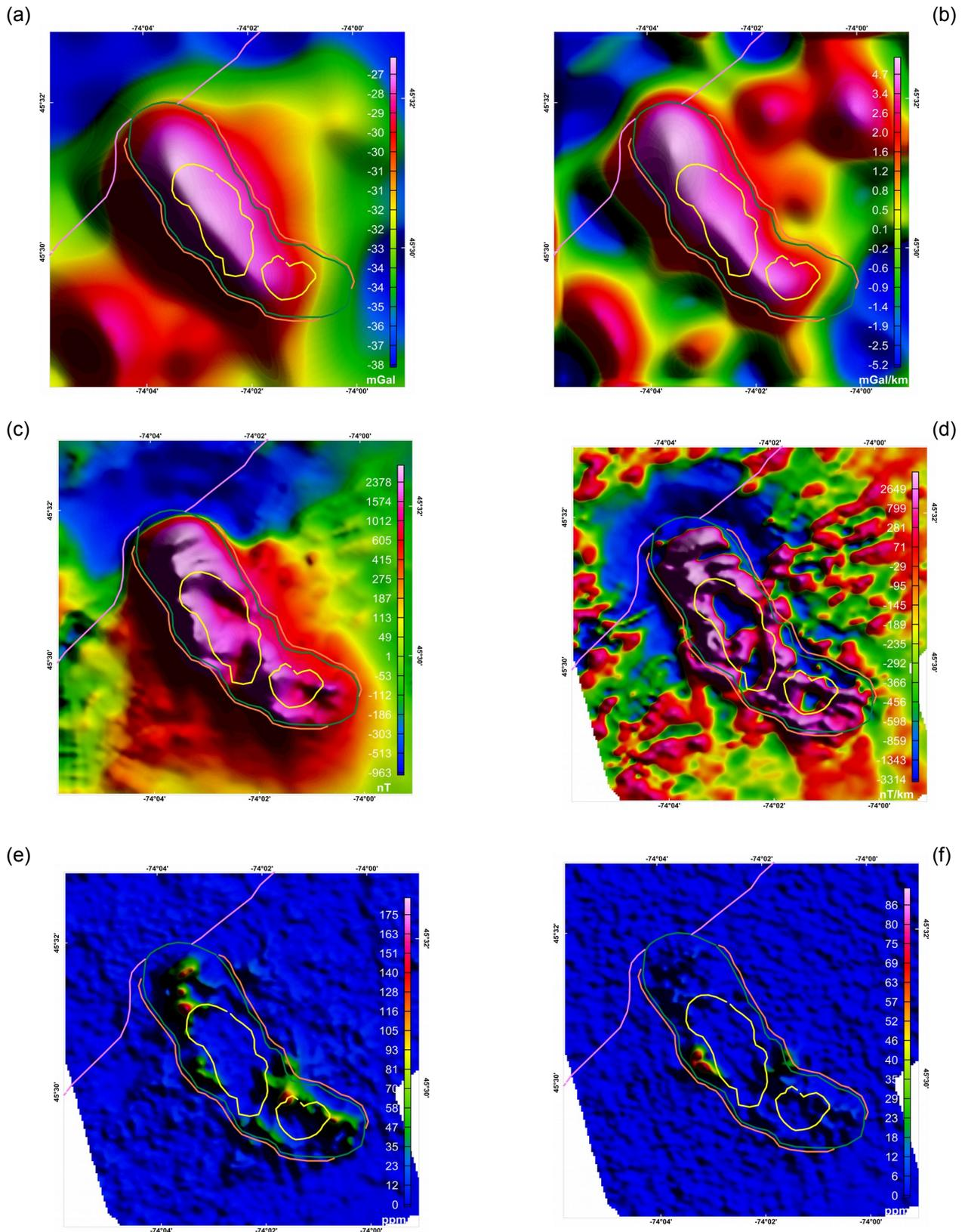
Figure 2 (a) Measured Bouguer gravity (b) first vertical derivative of Bouguer gravity (c) magnetic anomaly (d) first vertical derivative of the magnetic anomaly (e) Thorium equivalent concentration (f) Uranium equivalent concentration
