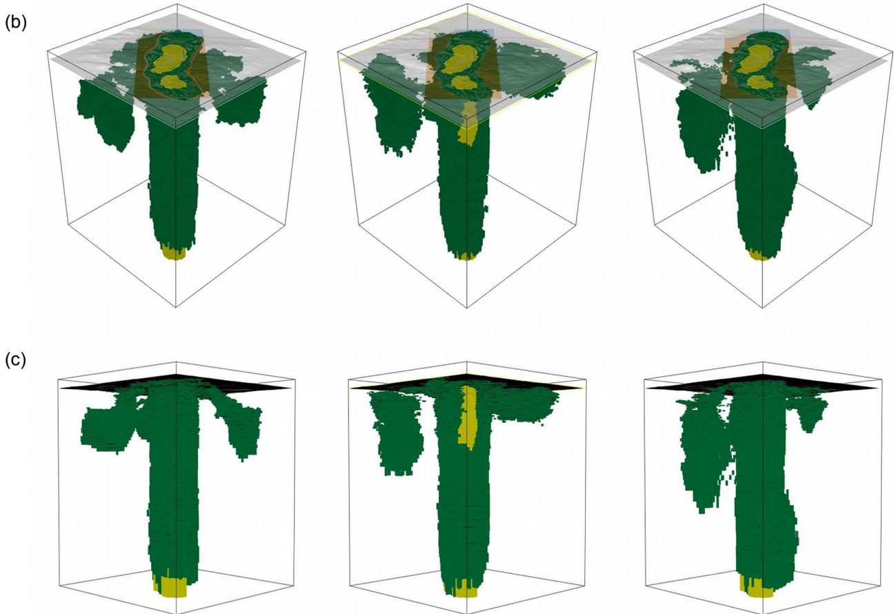
Figure 5 (a) Profile with observed data in red, gravity or magnetic only inversion in green and joint inversion in blue. (b) and (c) 3D views of inversion results showing silicate rocks in green and carbonates in yellow. Images on the left are from magnetic data only inversion, in the middle images from gravity data only inversion and images on the right are from joint gravity and magnetic data inversion. All figures have no vertical exaggeration.
