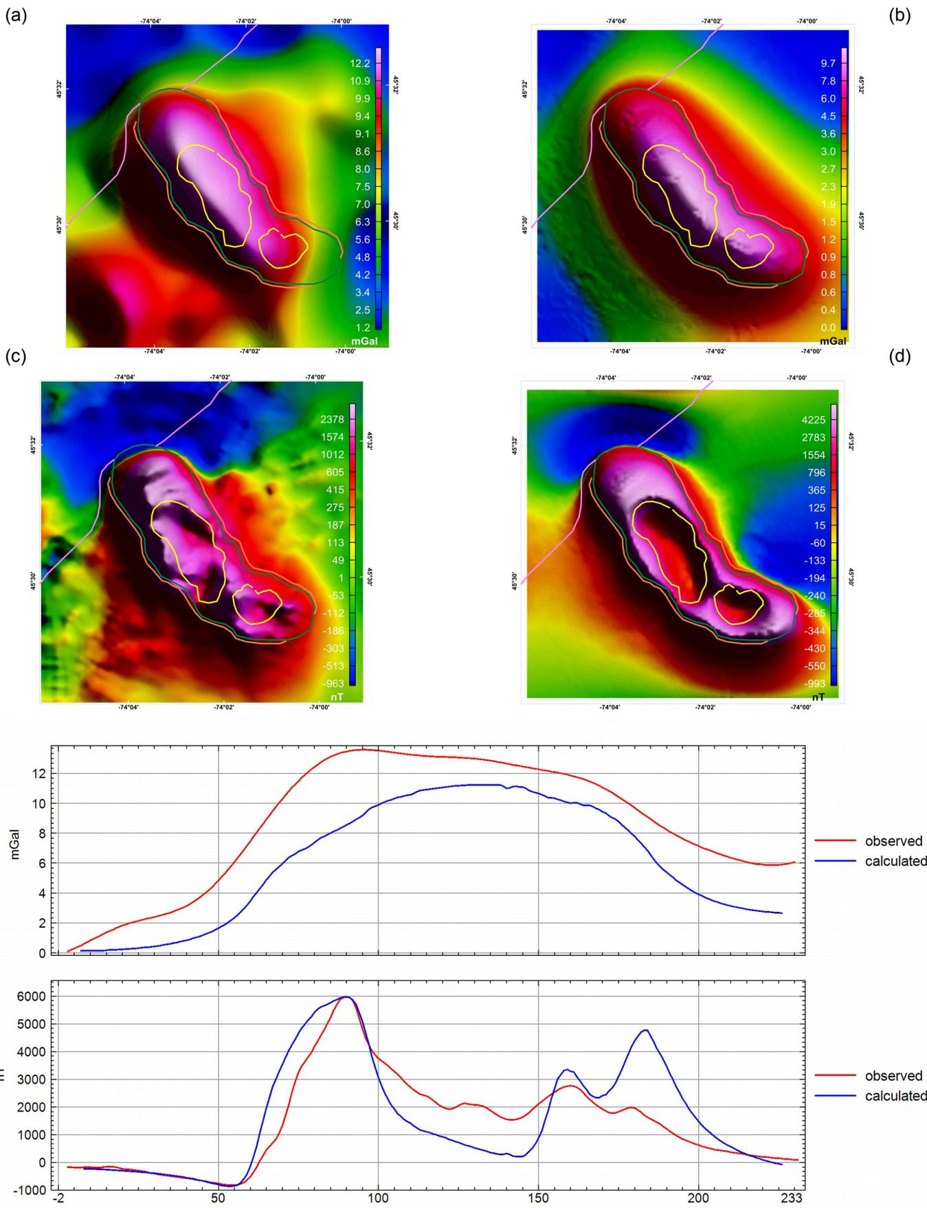
Figure 3 Pipe model: (a) measured Bouguer gravity (b) calculated Bouguer gravity (c) measured magnetic anomaly (d) calculated magnetic anomaly (e) gravity profile (f) magnetic profile
