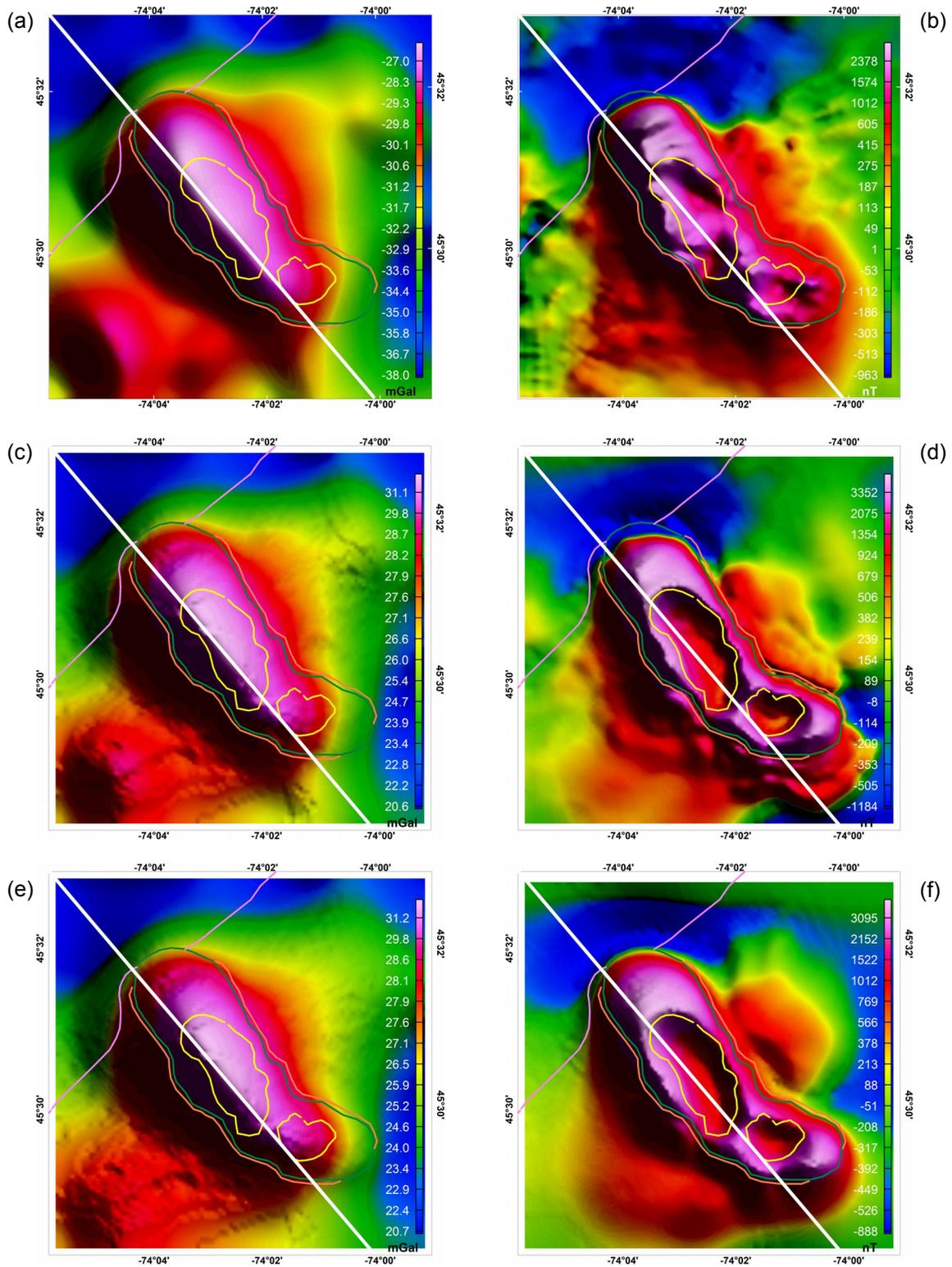
Figure 4 Inversion results grids. (a) Measured Bouguer gravity (b) measured magnetic anomaly (c) calculated Bouguer gravity from gravity only inversion (d) calculated magnetic anomaly from magnetic only inversion (e) joint inversion calculated gravity (f) joint inversion calculated magnetic anomaly. Location profile in Figure 5 marked.
