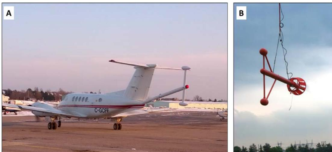
**Figure 6:** Airborne magnetic configurations for A: Fixed wing aircraft with tail plane having vertical gradiometer stinger; B: Helicopter suspended vertical gradiometer bird. Both systems are using Potassium optical pumped magnetometers.
