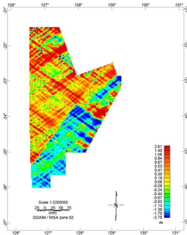
Figure 7. The difference in the terrain calculated from laser and GPS survey data from the Little Sandy Desert West Block compared to the SRTM.
