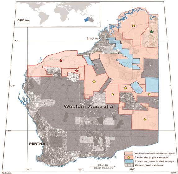
Figure 1. Location of the Geological Survey of Western Australia and Geoscience Australia’s large-scale reconnaissance gravity mapping project in Western Australia. Ground gravity stations are shown in grey, and airborne survey blocks are in colour. The airborne surveys flown by Sander Geophysics over several years are marked with a star (green for 2016, yellow for 2018, red for 2019).
