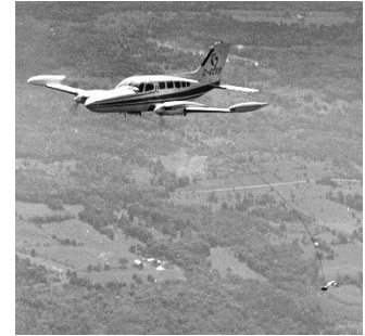
Cessna 402 towing "bird" with magnetometer in the early 1970s
