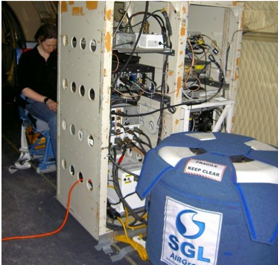
The AIRGrav system on-board the P-3 aircraft. Gravimeter (right), rack equipped with computers controlling the gravimeter and GPS receivers (center) and operator (left). Credit: Joël Dubé
