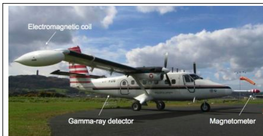
Fig. 4. The Tellus Border survey aircraft equipped with geophysical instrumentation.
