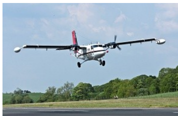
de Havilland DHC-6 Twin Otter equipped for multi-parameter surveys
